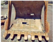
Original 400 BHN bucket liner held up for three months. Customer switched to manganal liner, floor, and sides which lasted a year and a half. Customer then rebuilt entire bucket out of manganal and reused original manganal liner which is still in use three years later.
