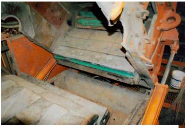
Manganal replaced tungsten carbide embedded AR 450 for impactor wear plates. AR 450 plates wore out in 3 months where the manganal plates have lasted 16 months showing light wear. The rotors pictured below were built up with Stulz manganese XL welding electrodes.
