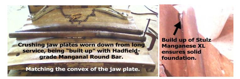
Welder tack-welded and bent 2" round stock to jaw plate. Built up between round bar and plate and skip-welded edges all with Stulz XL.
