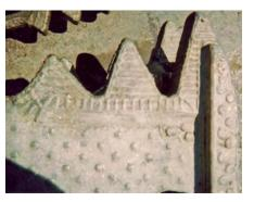
Manganal teeth fabricated for processor before (shown to the left) demolition of Adams Mark Hotel in Philadelphia. Processed 50,000 yards of concrete. Very little wear at end of job (shown to the right).
